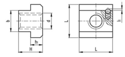
b -0.1 -0.3 = 12 d = M10= 14 Н = 7 h1 L = 18 11 = 0.7T-slot width DIN 650 = 12
